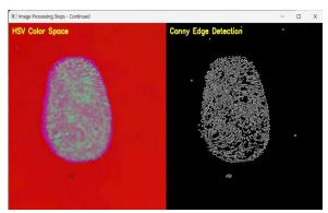
Fig.3- Enhancement of image using HSV colour space and canny edge detection.
